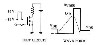
$$\begin{aligned} R_G &= 25~\Omega \\ V_{DD} &= 90~V,~L = 25.5~mH \end{aligned} \quad E_{AS} &= \frac{1}{2} \cdot L \cdot I^2 \cdot \left( \frac{B_{VDSS}}{B_{VDSS} - V_{DD}} \right) \end{aligned}$$
