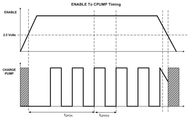
Figure 5: Timing Diagrams for VDD to RESET and Enable to Charge Pump Active.
