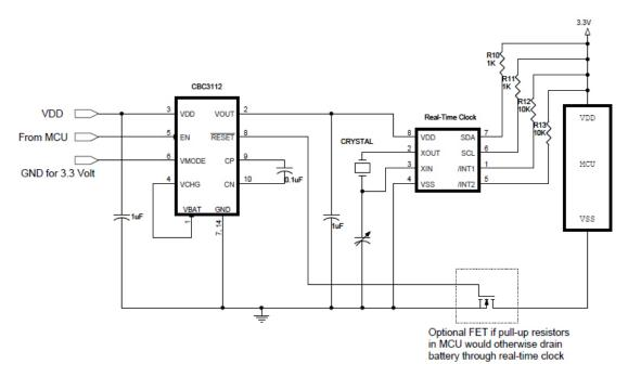
Figure 10: EnerChip CC Providing Real-Time Clock Backup Power
