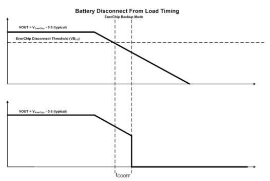
Figure 4: EnerChip CC Switchover and Disconnect Timing Diagrams
