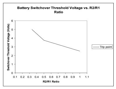
Figure 8: Mode 2 Resistor Selection Graph
