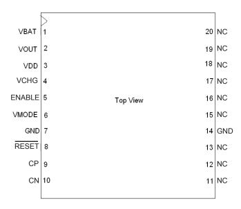
Figure 3: EnerChip CC CBC3112 Package Pin-out
