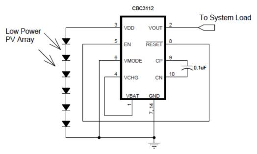
Figure 13: Implementing Energy Harvesting with the EnerChip CC
